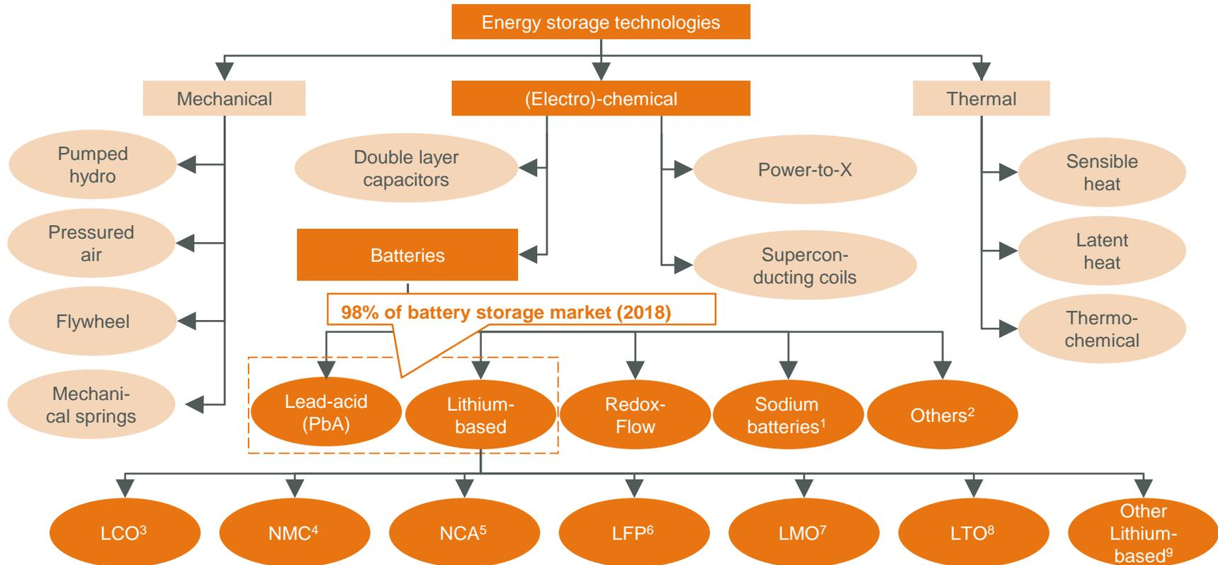
Source: Apricum analysis; 1) Includes NaS, NaNiCl and Sodium-ion batteries; 2) E.g., Zinc-Air, liquid metal batteries, NiMH, NiCd; 3) Lithium Cobalt Oxide; 4) Lithium Nickel Manganese Cobalt Oxide; 5) Lithium Nickel Cobalt Aluminum Oxide; 6) Lithium Iron Phosphate; 7) Lithium Manganese Oxide; 8) Lithium Titanate; 9) Including Li-metal, Li-S and Li-air batteries
