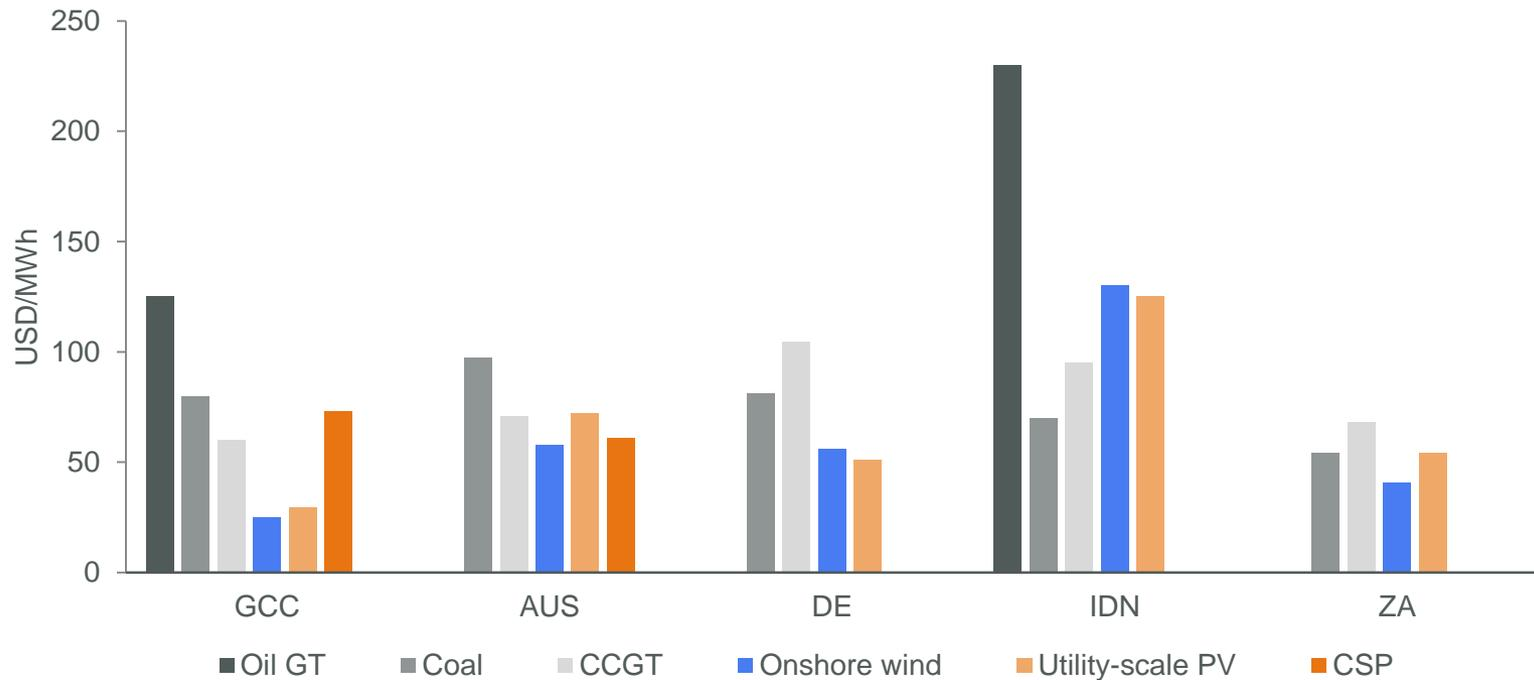
GCC= Gulf Cooperation Council countries; AUS = Australia; DE = Germany; IDN = Indonesia; ZA = South Africa; GT= Gas turbine; CCGT = combined cycle gas turbine; PV = photovoltaic; CSP = concentrated solar power
